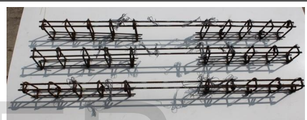
Fig. 4. A view of TMT reinforcement cages
